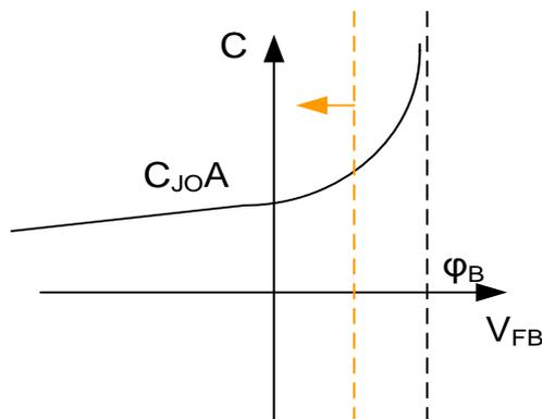
$$C = \frac{C_{J0} A}{\left(1 - \frac{V_{FB}}{\phi_B}\right)^m}$$
