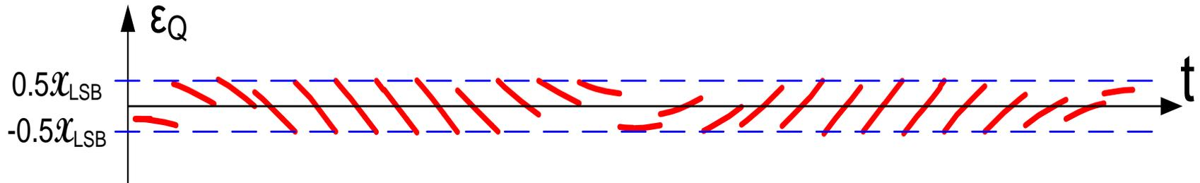
For low  $f_{\text{SIG}}/f_{\text{CL}}$  ratios, bounded by  $\pm 0.5 X_{\text{LSB}}$  and at any point in time, behaves almost as if a uniformly distributed random variable
