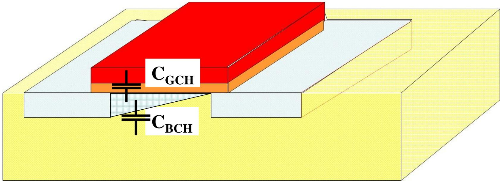
Note: Since the channel is an extension of the source when in saturation, the distributed capacitors to the channel are generally lumped to the source node
