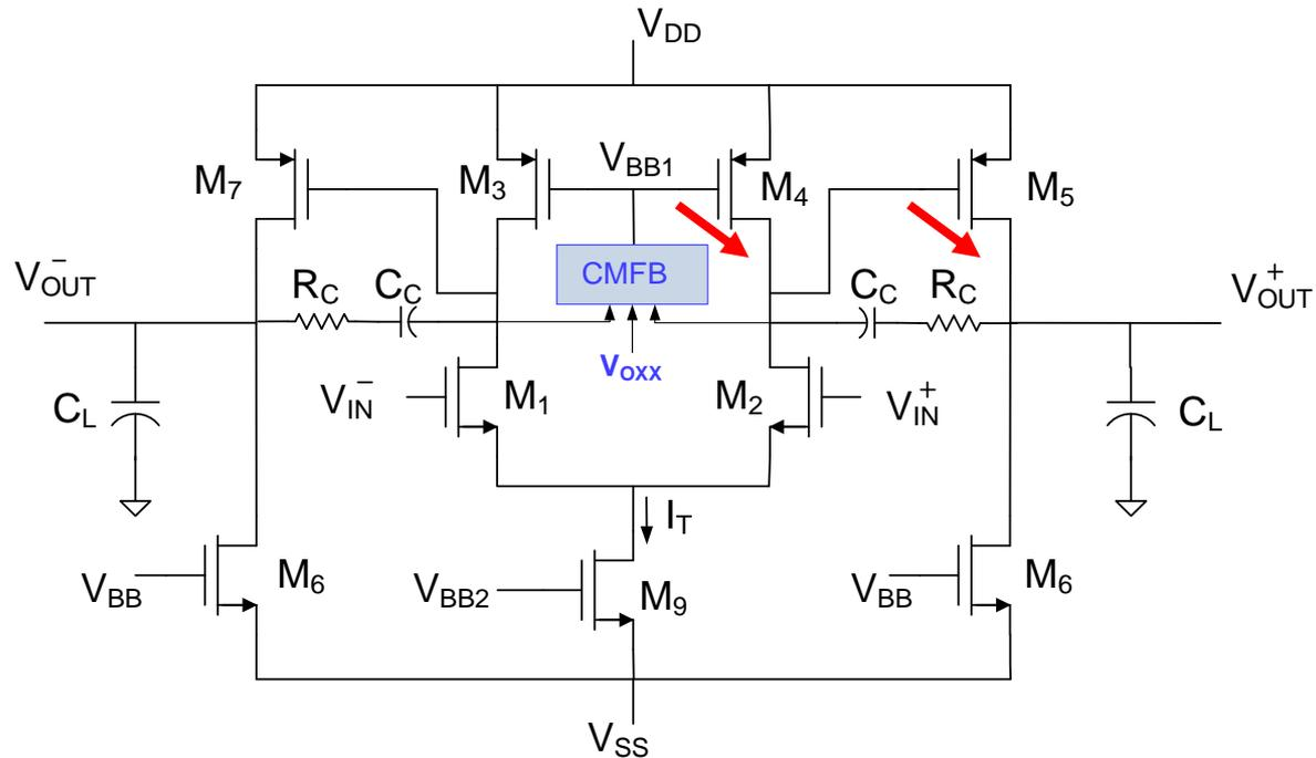
Must have negative feedback to control biasing of first stage of Op Amp
