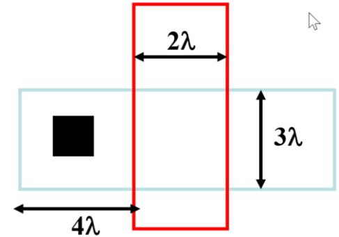
$$\text{Gate-Channel Capacitance} = 6\lambda^2 \times 2.47\text{fF}/\mu^2 = \mathbf{1.33\text{fF}}$$
