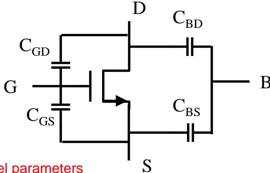
$C_{BOT}$  and  $C_{SW}$  are model parameters
