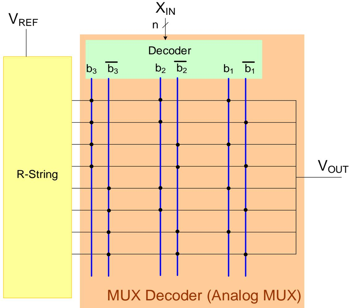
MUX decoder is comprised of analog AND gates
