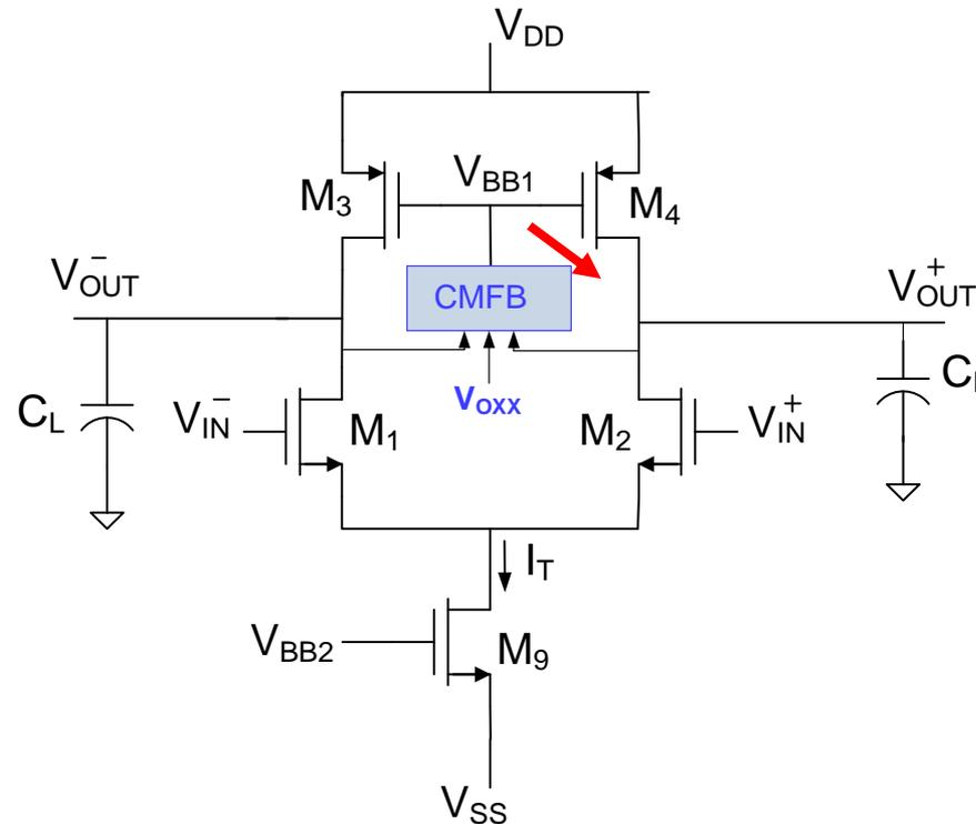
Must have negative feedback to control biasing of first stage of Op Amp
