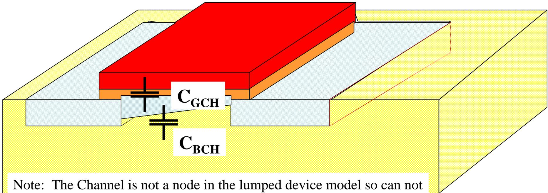
Note: The Channel is not a node in the lumped device model so can not directly include this distributed capacitance in existing models
